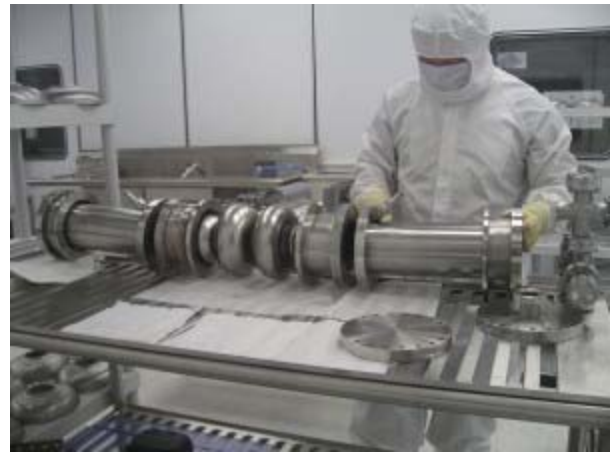
Niowave employee cleans niobium cavity. Image: Niowave
